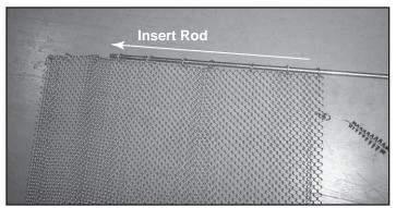
Figure 8.11 Insert Rod into Firescreen
